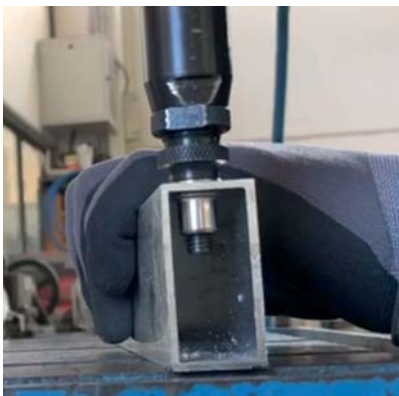
3. Pull the trigger, the machine will stop automatically.
