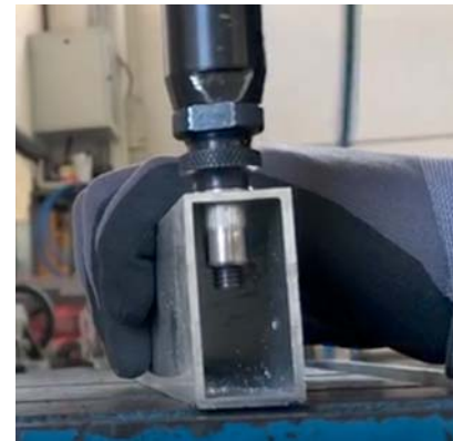
2. Include the threaded insert using a pneumatic/electric riveting tool.
