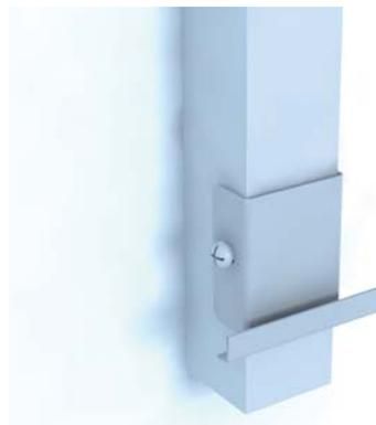
2. Apply the first row of ZCLW-KK2806 clips at the bottom with self-drilling screws.
