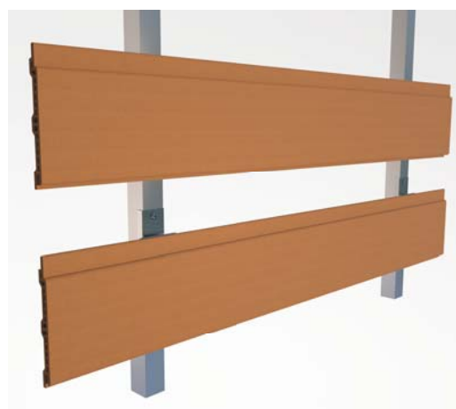
6. Repeat as described from step 3 up to the top to complete the cladding
