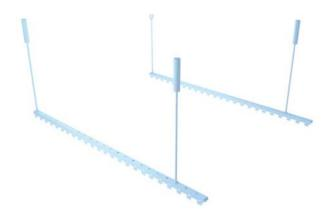
1. Fix the ZSSW-LG9637V bars directly to the ceiling using screws and wall plugs suitable for the type of support, or lower the structure with suitable hangers.
